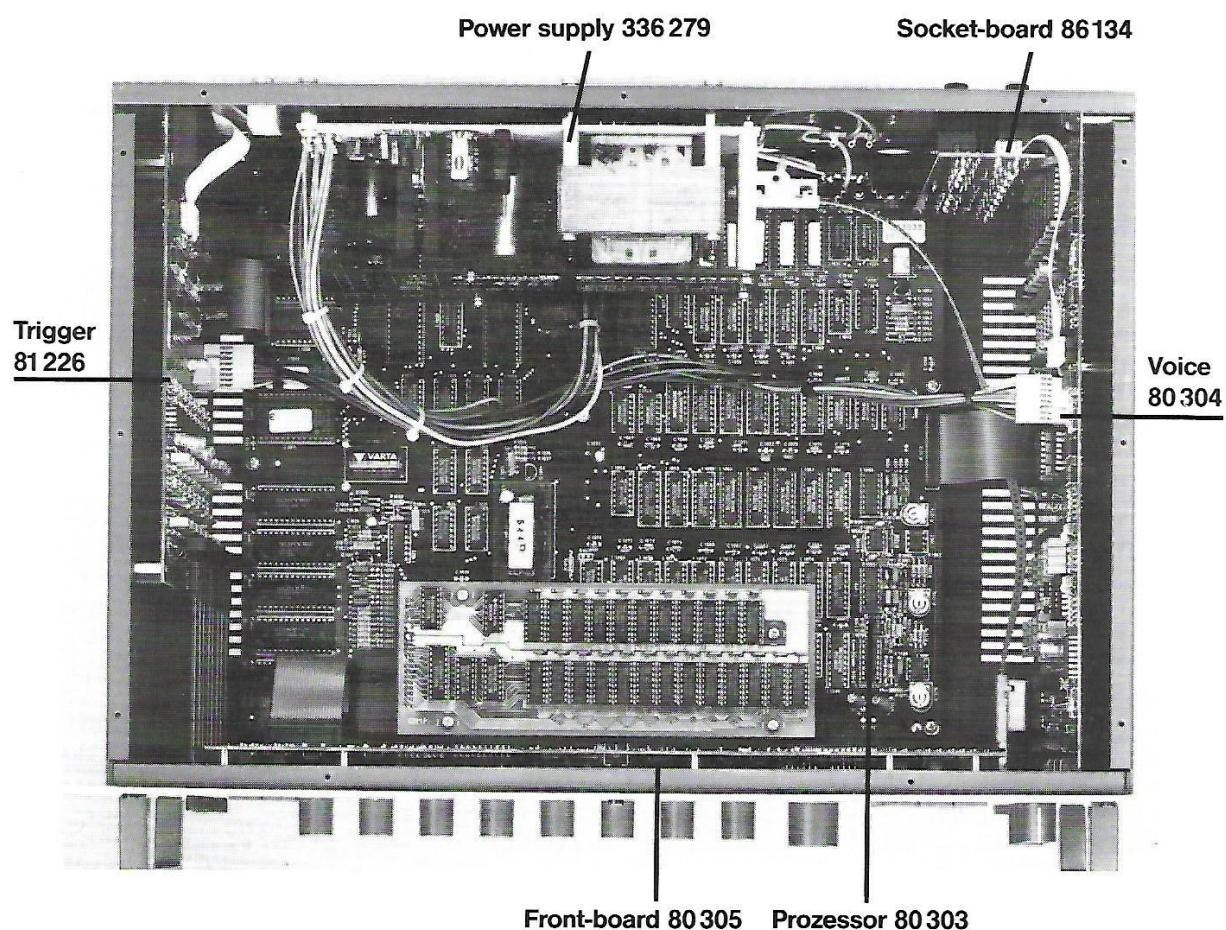
Faults in the digital section of the processor board can in most cases only be detected with expensive measuring instruments (68009 emulator, 16-channel logic analyzer and 100 MHz oscilloscope). It is therefore advisable to return this board to the factory for repair. Please enclose an exact fault description.
